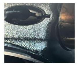
The engine block must be inspected for excessive wear on the cam-follower cylinders and camfollower key guides and verified serviceable by the supplier for warranty purposes.
