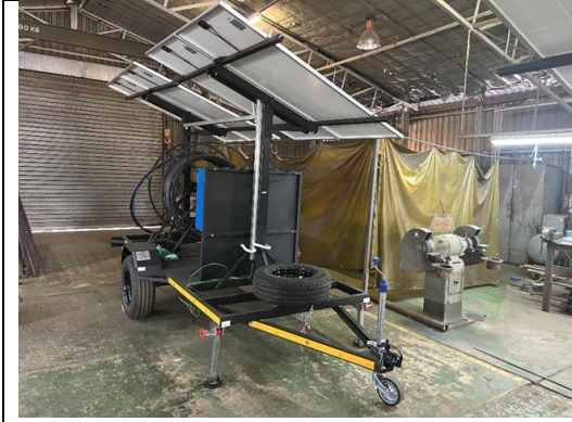
Figure 1: The Mobile solar trailer consists of the following as seen in the picture; Electrical enclosure box, Spare wheel, Jockey wheel, Hose reel, Steel pump & Adjustable solar panels.
