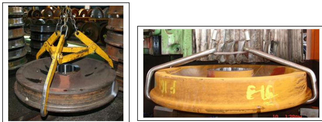
Figure 7: Wheel centre lifting devices – horizontal clamping.
