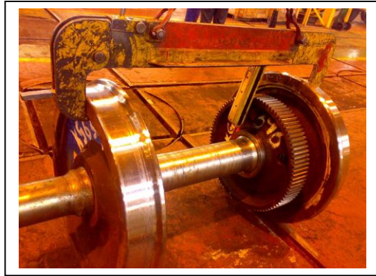
Figure 1: Wheelset lifting device as per drawing a) TWK13171 and b) TWK16219 .
