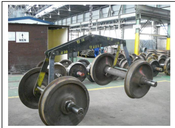
Figure 2: Double wheelset lifting device as per drawing.
