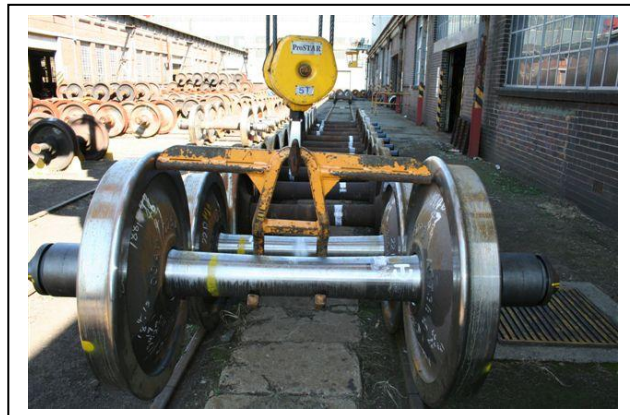
Figure 3: Wheelset lifting device as per drawing.
