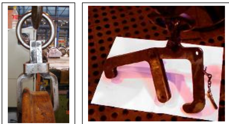
Figure 6: Wheel centre lifting devices – vertical clamping.
