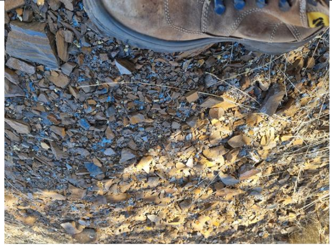
Figure 4: Asbestos containing discard with loose fibres.
