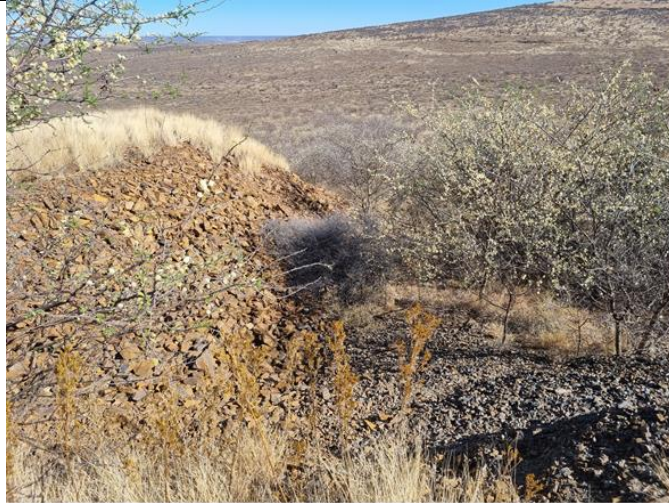
Figure 3: Partially vegetated Asbestos dump with fibres that can easily be carried away by water or wind.
