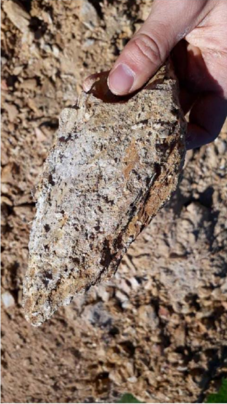
Photo 5 – Close-up view of highly weathered phyllites.
