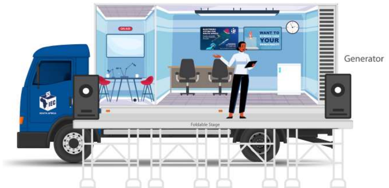
A side view illustration of the truck, showing the interview room, workstation desk, and the foldable stage. The generator is located at the back of the truck and can be accessed from the outside.
