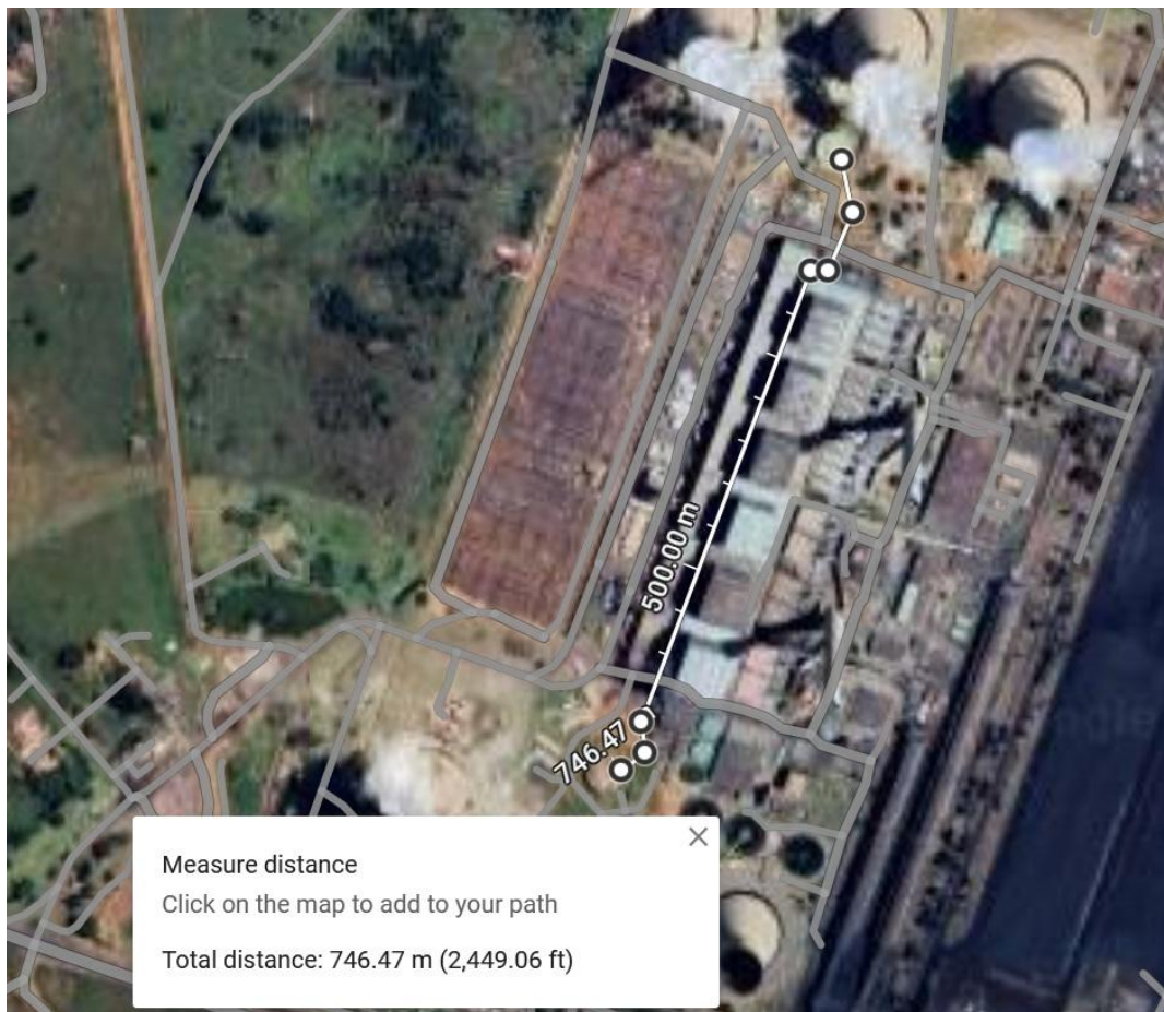
Figure 1: Approximate cable route distance between Duvha North and South Pumphouse is 746 m
