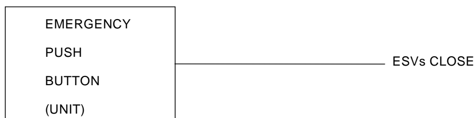
Figure 4.3.17.1 — Emergency push-button tripping logic
