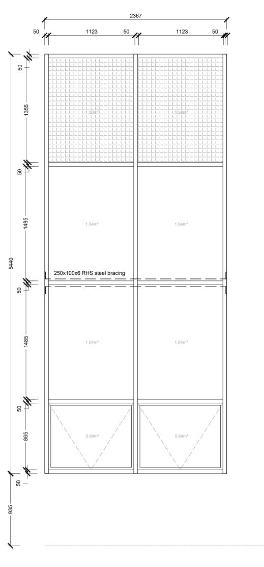
CWType P Crealco Facade 60 or eq. approved aluminium pressure glazed drained facade system, incl top hung casement insert window, per layout.
