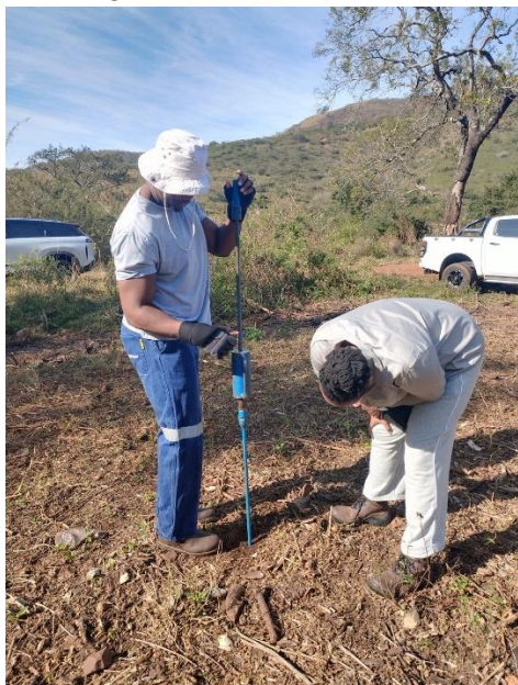
Figure 13: Image of DCP Test at position X 5
