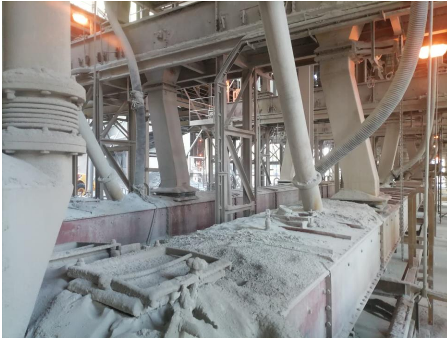
Figure 8: Collector Conveyors Arrangement
