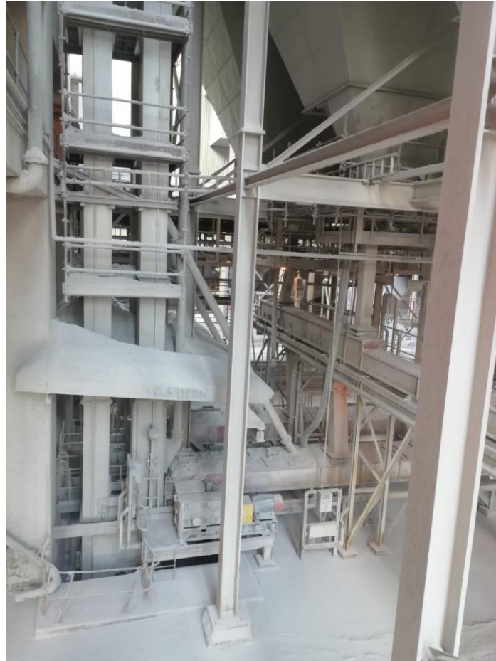
Figure 9: Bucket Elevator Arrangement
