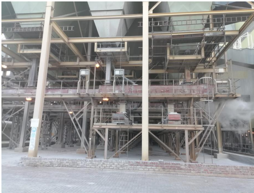
Figure 1: Matimba's Hopper & Collector conveyors Layout
