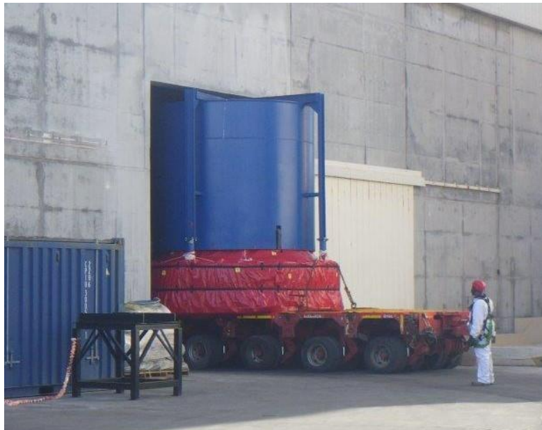
Figure 7: Unit 2 head entering the Low-Level Waste Building storage
