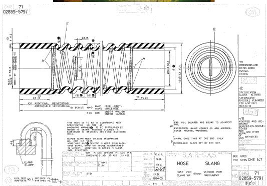
13.5 M00043956 - Hose, non-metallic; type brake coupling; users' description: item a20 ref 3 (6e, 6e1, 9e) item a25 ref 3 (5m2a) 15-16-01 fig 1 it 3 (5m2a, 6e1, 7e, 7e1) class
