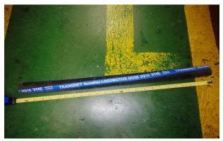
13.6 M00064226 - Hose, non-metallic; type vacuum, length max 470 mm, material rubber, nominal diameter 20.6 mm; old material no 071007105, equipment used on wagon specification number cme 147/1992/july
