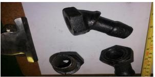
13.4 M00023075 - Hose, non-metallic; type vacuum, length max 640 mm, material rubber, nominal diameter 59.3 mm; users' description 50mm allied item 71/012564 (assembly), equipment used on wagon specification number cme 147/1992/july.
