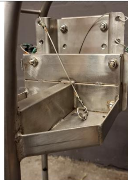
Backplate supporting pressure housing made of 3mm 316 marine grade stainless steel.
