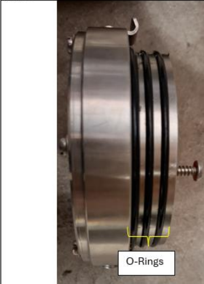
3 x O-rings in housing lid to allow no water to enter camera housing
