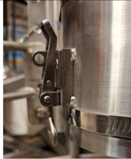
Stainless steel solid hinge clamps on housing
