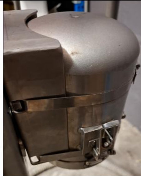
Back plate to secure housing in position.
