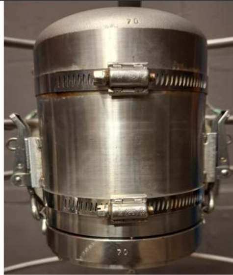
Stainless steel clamps to secure housing to back plate.
