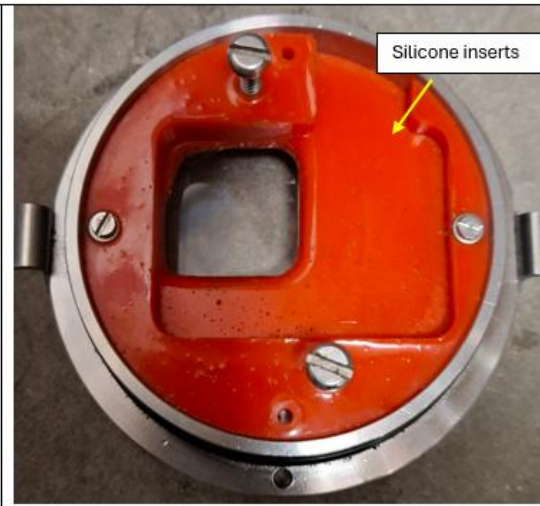
Silicone inserts to house GoPro 8 and GoPro 10 action camera's. Secured to lid with 316 grade screws.
