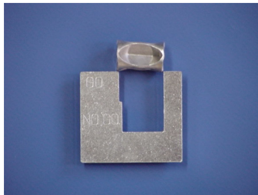
Figure 3: The test slug does not fit into the gauge, indicating that the crimper is operating at too high a pressure
