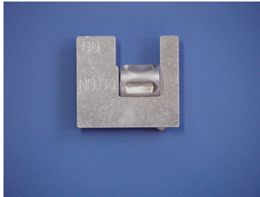
Figure 4: The test slug fits in the NO-GO part of the gauge, indicating that the crimper is operating at too low a pressure
