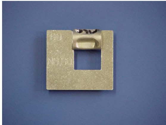
Figure 2: The test slug fits in the GO section of the gauge indicating that the crimper is operating correctly
