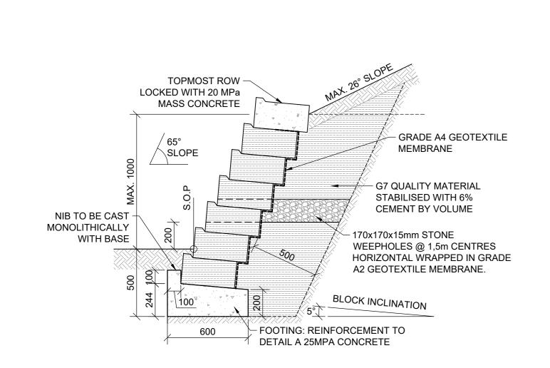
TYPICAL SECTION SHOWING DRY-STACK RETAINING WALL (>0m TO 1m EXPOSED HEIGHT)
