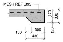
**SLAB EDGE THICKENING DETAIL**
