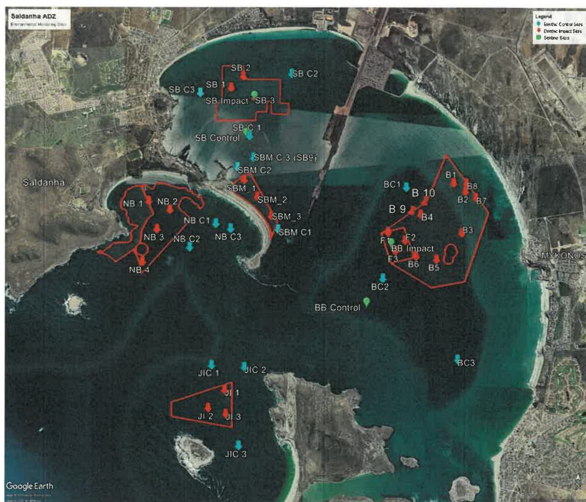
Figure 1: Map of sampling stations for the Saldanha Bay Aquaculture Development Zone showing the benthic chemical (sulphide & redox), sediment (organics, PSD and metals), macrofauna and sentinel (near bottom DO and temperature) sites.
