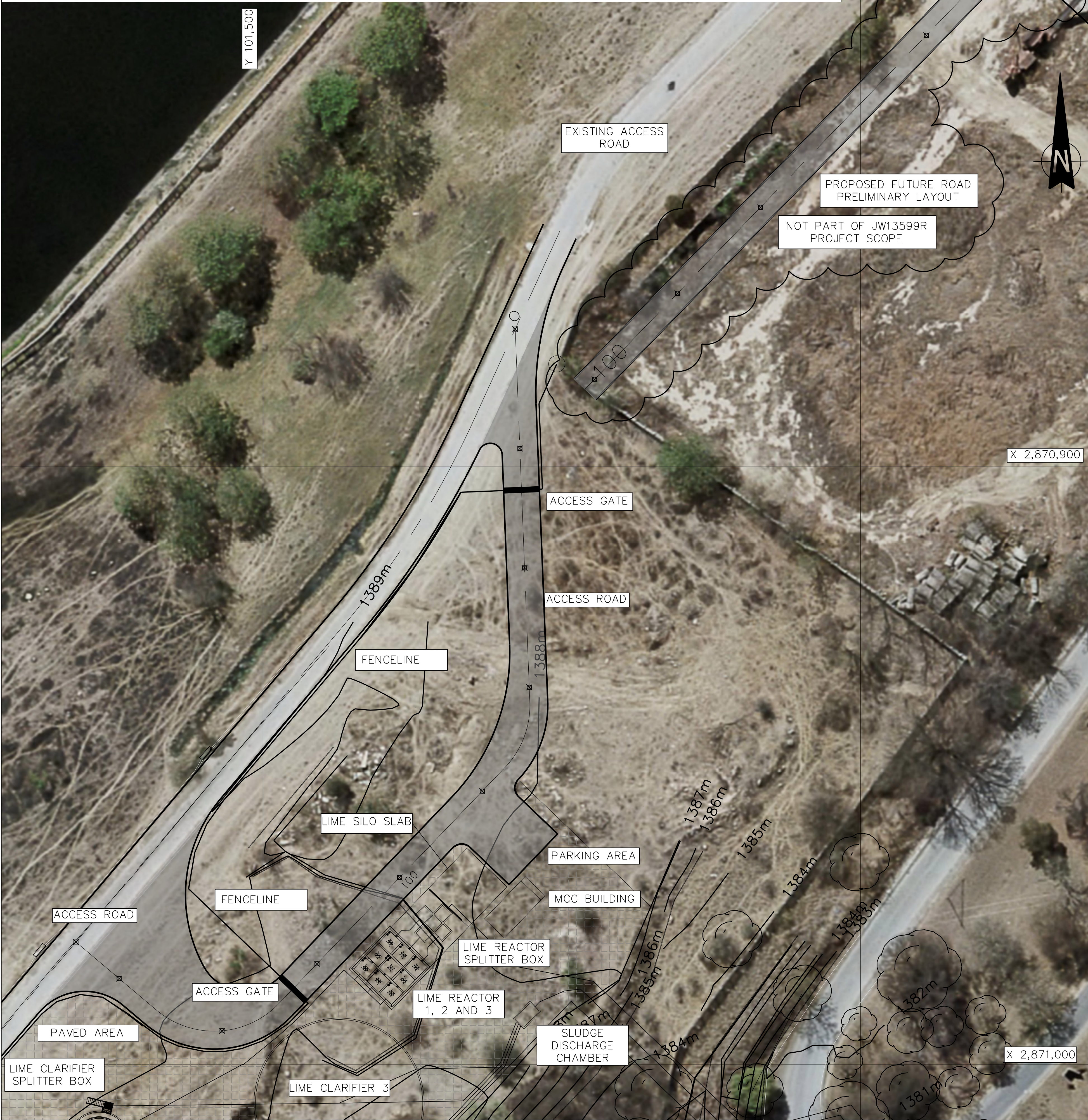
ACCESS ROADS – LAYOUT PLAN SCALE 1:500
