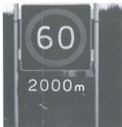
Detail 15.28.2 Boxed Fibre Optic VMS Composition
