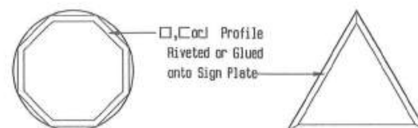
Detail 15.22.4 Perimeter Bracing Only
