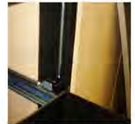
Locking mech integral part of anti-tilt mech and runner design.
