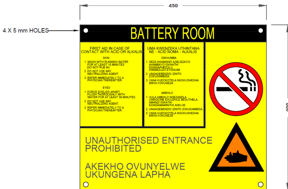
Figure 43 – Screen printed chromadek “Battery room” sign
