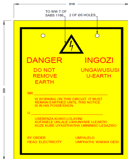
Figure 29 – Hardboard “Danger do not remove earth” sign
