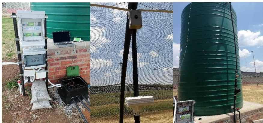
Fig 5: An automated irrigation system and a pump covered/protected in a black plastic frame (A), with the climate sensor in the minitunnel (B) and a water tank (C).
