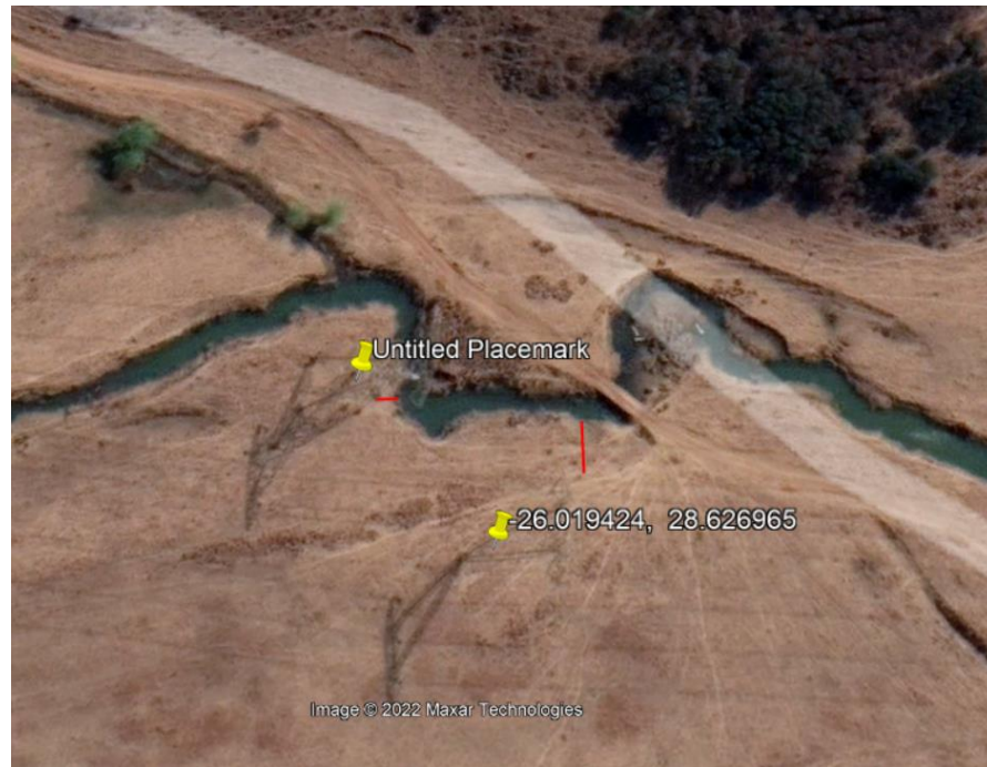
Figure 12: Erosion on the stream embankments towards the foundations (Google Earth imagery)
