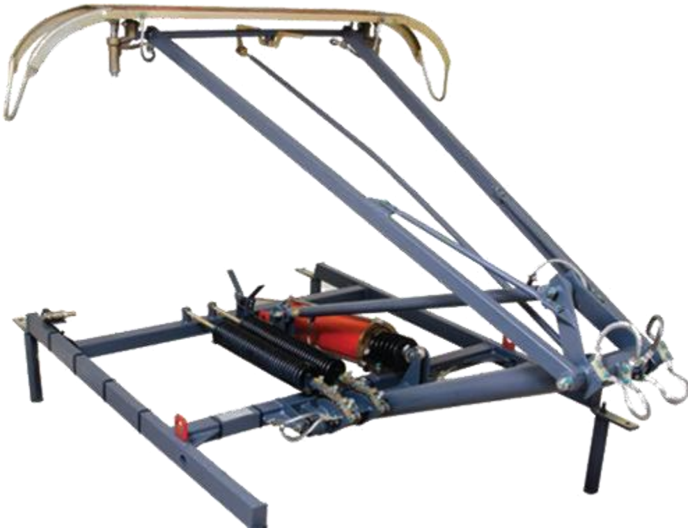
Figure 1: Pantograph with Carbon Strip (ADD/DDU)
