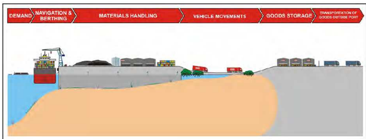
Figure 7: Conceptual model of a port and the main activities which can be affected by climate change
