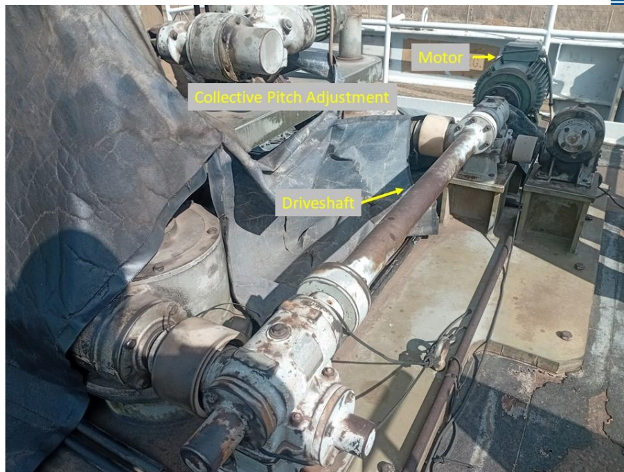
Figure 2: Collective Pitch Adjustment
