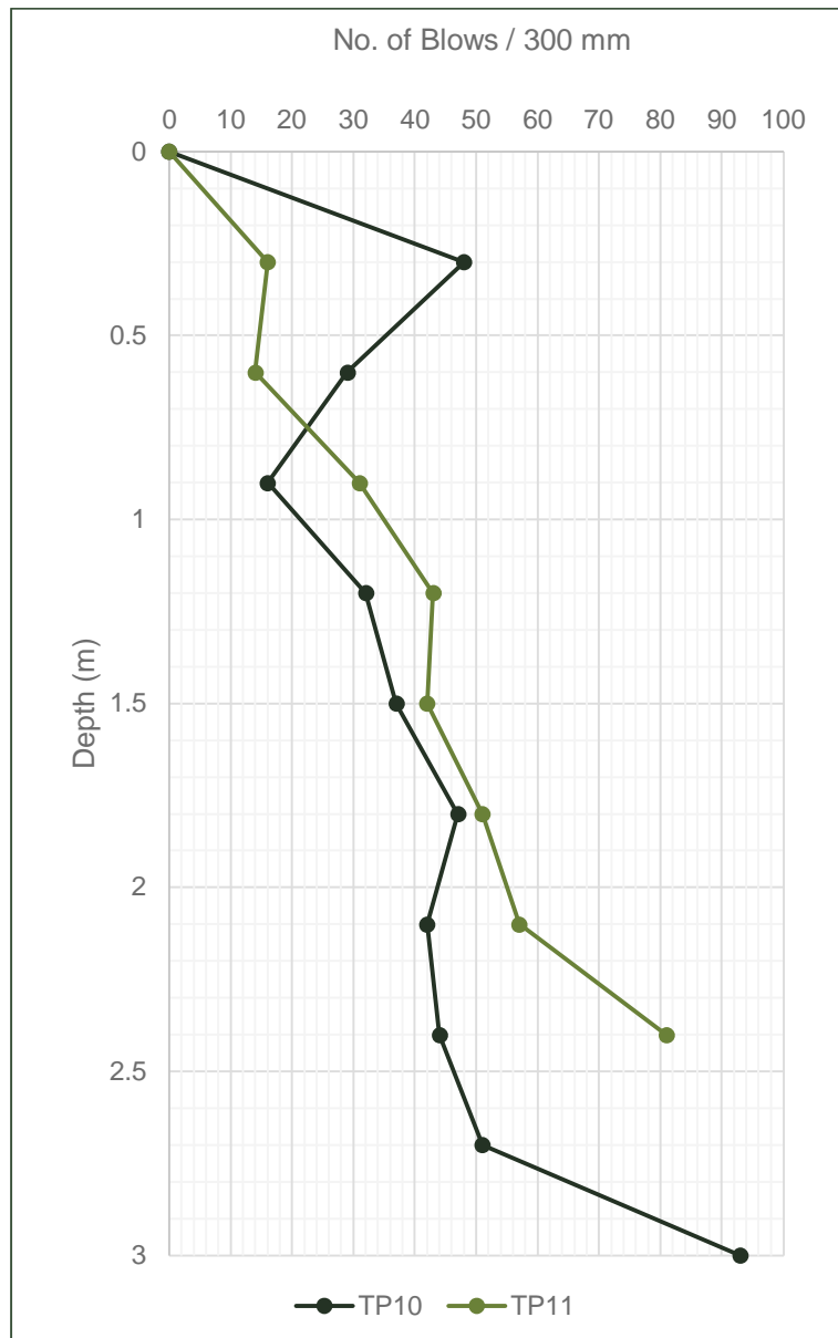
Figure 4-13: Second Class Water System DCP Test Results
