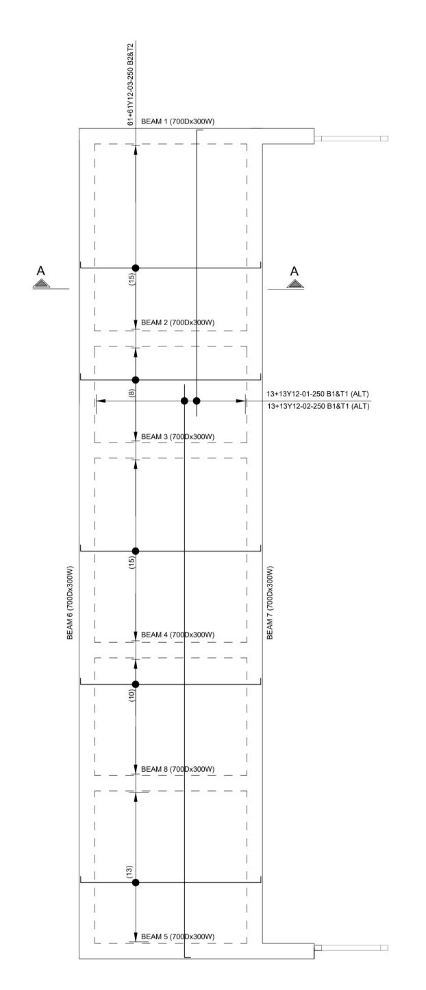
OFFICE BLOCK FOUNDATION REINFORCEMENT LAYOUT SCALE 1:50
