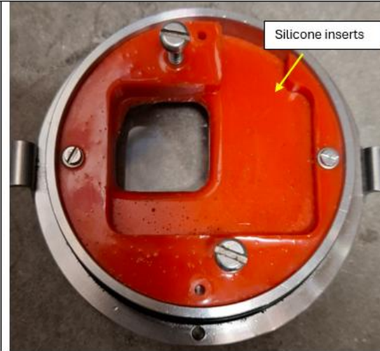
Silicone inserts to house GoPro 8 and GoPro 10 action camera's. Secured to lid with 316 grade screws.
