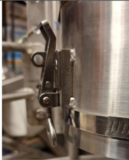
Stainless steel solid hinge clamps on housing
