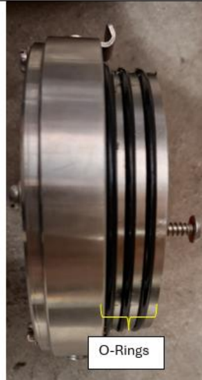
3 x O-rings in housing lid to allow no water to enter camera housing
