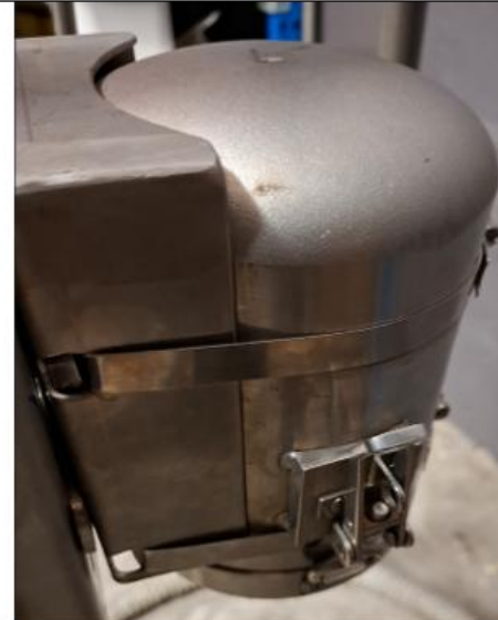
Back plate to secure housing in position.
