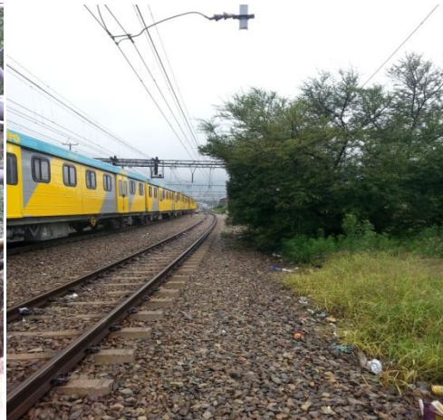
Figure 2: Trees encroaching on railway lines
