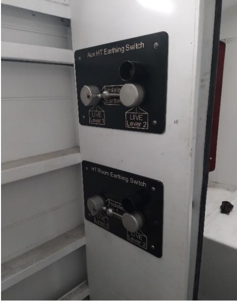
Fig 3- Earthing switches on a coach
