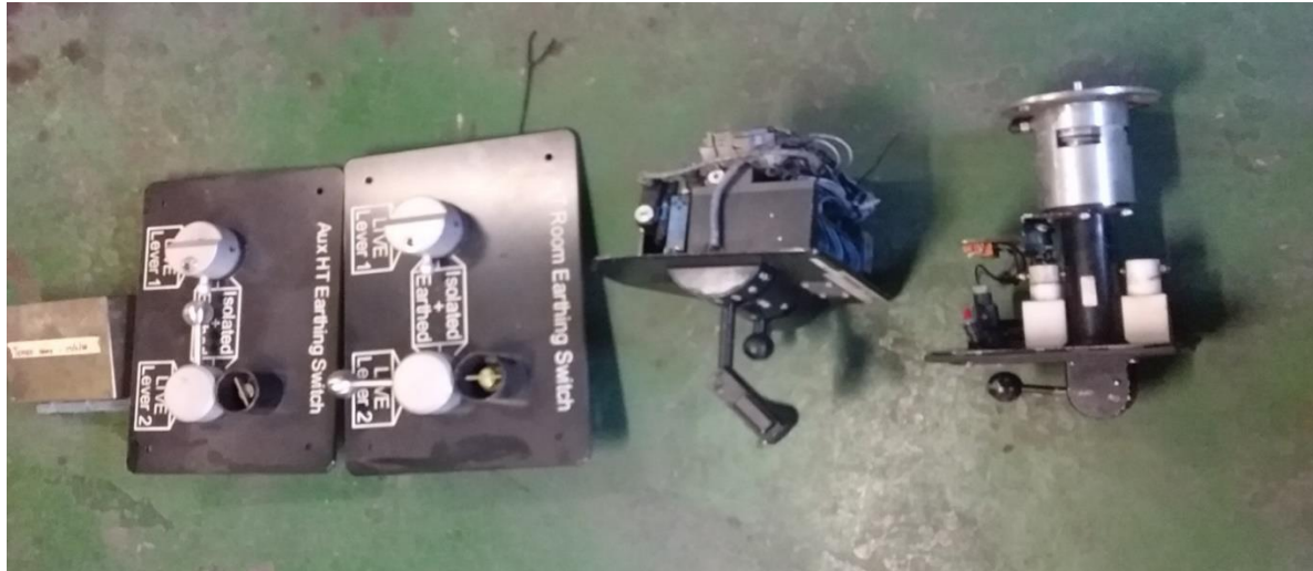
Vigi-drive, Earthing switches, Master controller and Emergency brake valve
