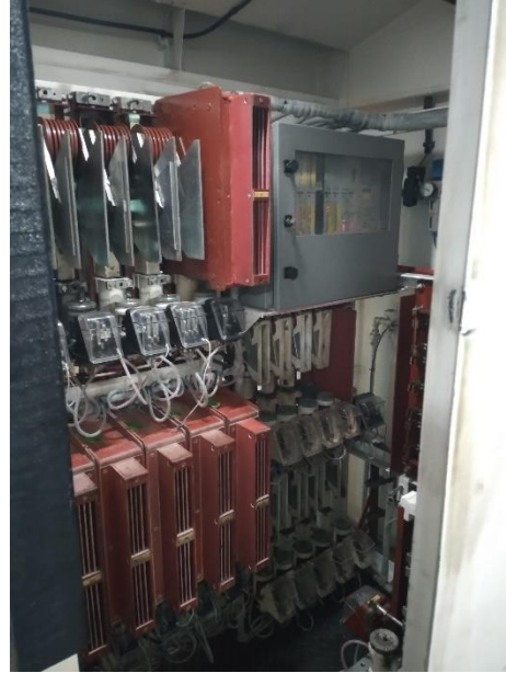
Fig 4– High tension compartment on a coach
