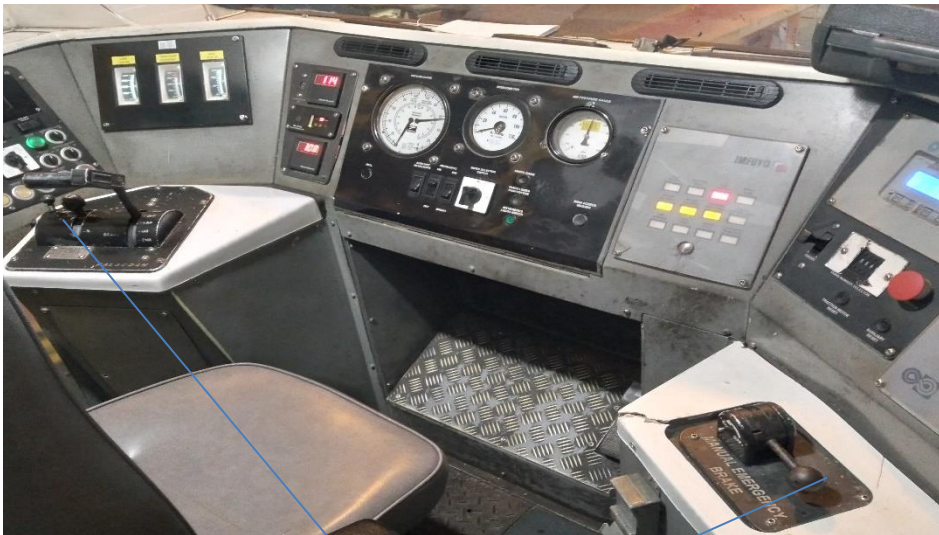
Fig 2 – Master controller (MC) and Brake valve (BV) located on a coach
