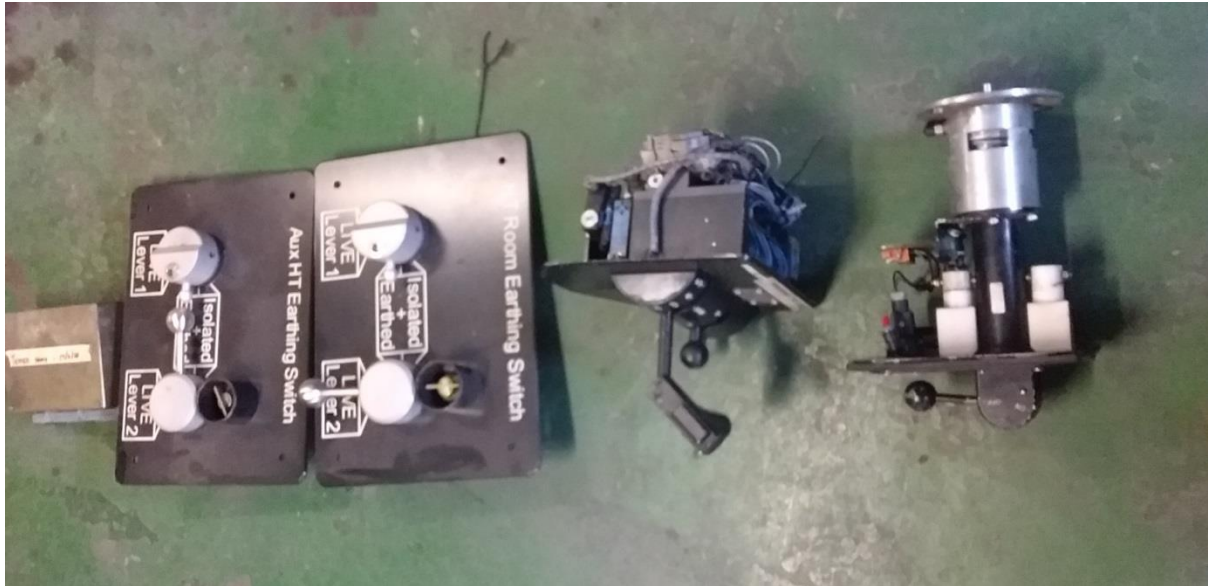
Fig 1 – Vigi-drive, Earthing switches, Master controller and Emergency brake valve
