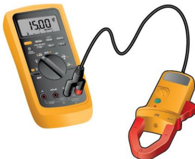
Figure 4: Clamp meter used with the multimeter.
