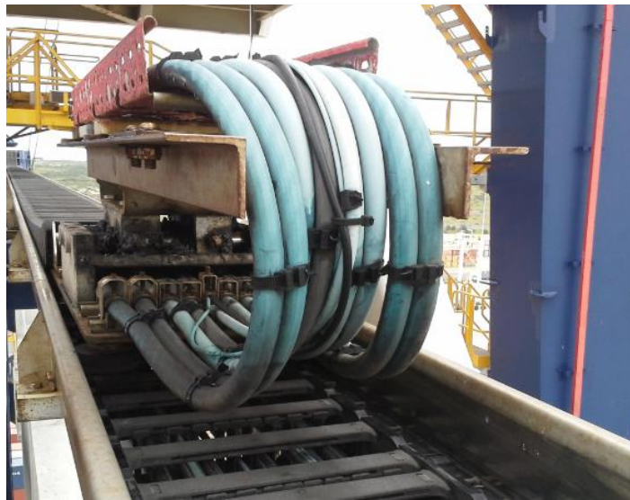
Figure 2: Floating head to be refurbished
