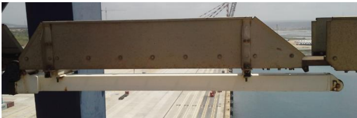
Figure 3: Link/hinge arm and pin location to be repaired
