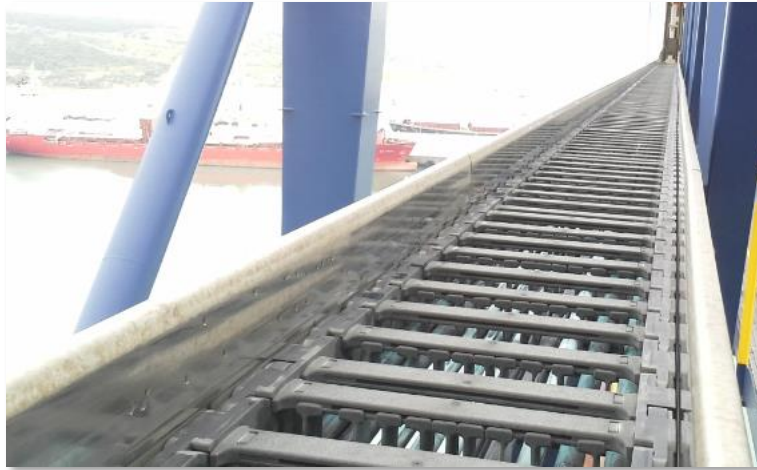
Figure 4: Entire trough and link arms to be aligned
