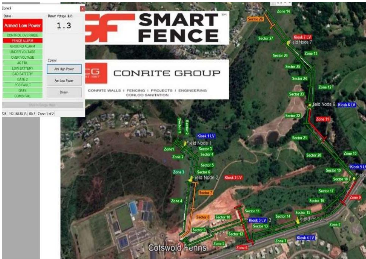
Figure 2: This is a typical example of a full perimeter system set up. When alarms are triggered then the system alarms in red and has a live voltage reading . Alarms are to have a full reporting system to allow for QA/ QC interfacing .
