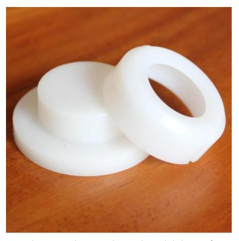
Designed to accommodate 25 mm diameter discs with thicknesses of: 0.4 mm binding layer, 0.8 mm diffusive layer and a 0.14 mm filter membrane
