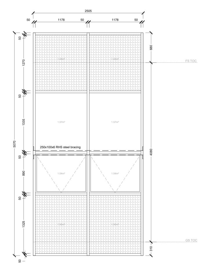
CWType C Crealco Facade 60 or eq. approved aluminium pressure glazed drained facade system, incl top hung casement insert window, per layout. Casement sash 1500 x 1200mm max capacity. Mullions in 160mm depth section, code W58433 with Lx 484 Fixing suitable for fixing to concrete / brickwork reveals.
