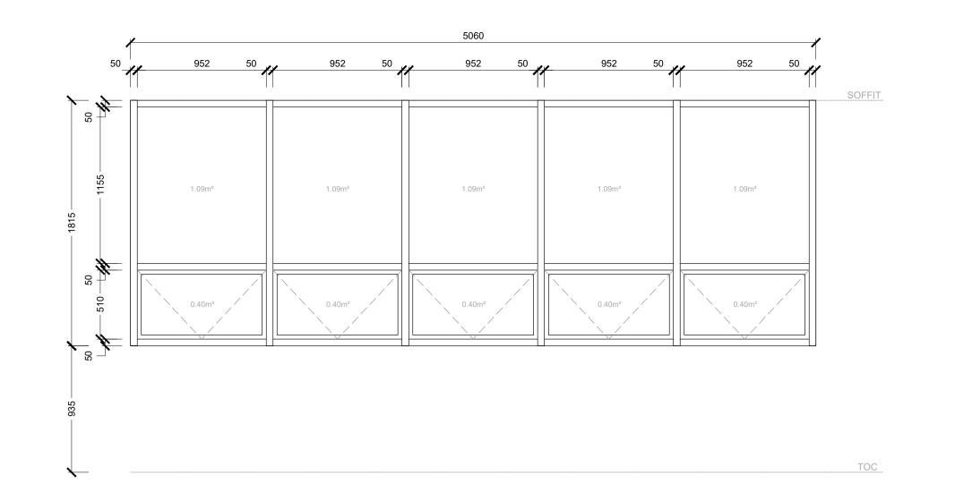
CWType A Crealco Facade 60 or eq. approved aluminium pressure glazed drained facade system, incl top hung casement insert window, per layout.
