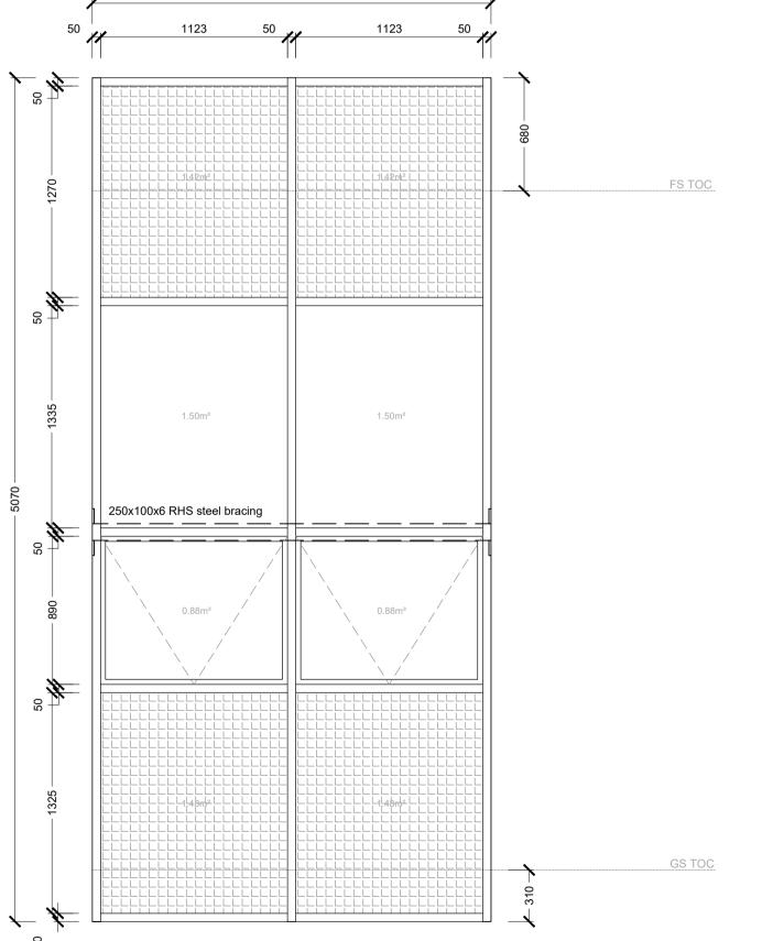
CWType E Crealco Facade 60 or eq. approved aluminium pressure glazed drained facade system, incl top hung casement insert window, per layout. Casement sash 1500 x 1200mm max capacity. Mullions in 160mm depth section, code W58433 with Lx 484 Fixing suitable for fixing to concrete / brickwork reveals.
