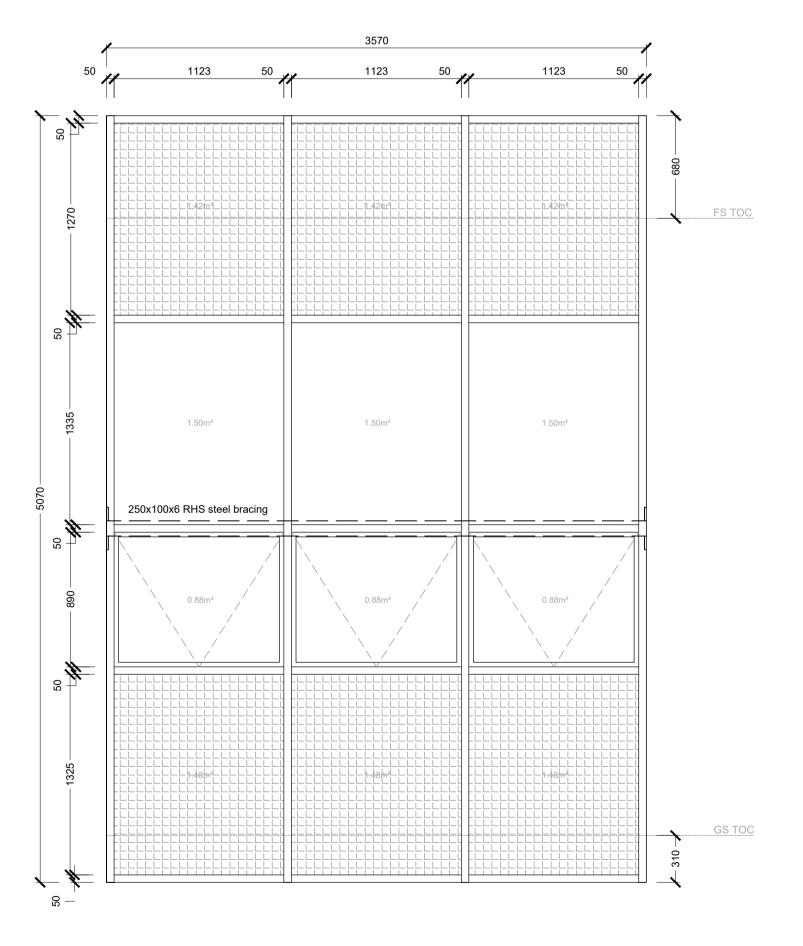
CWType D Crealco Facade 60 or eq. approved aluminium pressure glazed drained facade system, incl top hung casement insert window, per layout. Casement sash 1500 x 1200mm max capacity. Mullions in 160mm depth section, code W58433 with Lx 484
