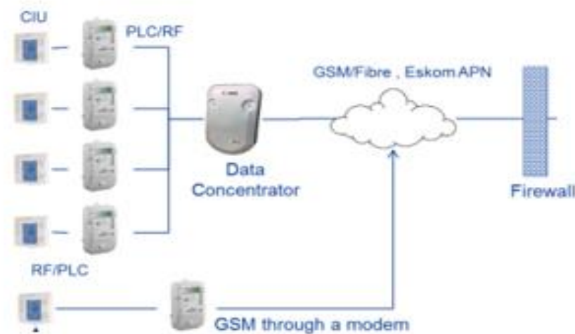
Figure 1: Simplified Smart Meter Architecture
