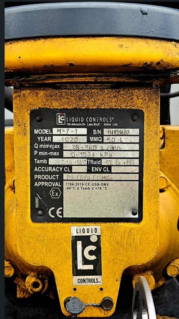
Pier 1 Mobile Bowser Truck - Flow Meter NamePlate.jpg
