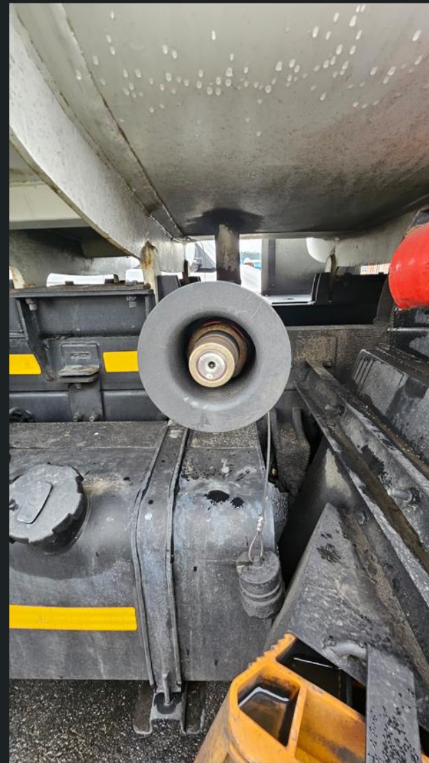
Pier 1 Mobile Bowser Truck - Filling Point.jpg
