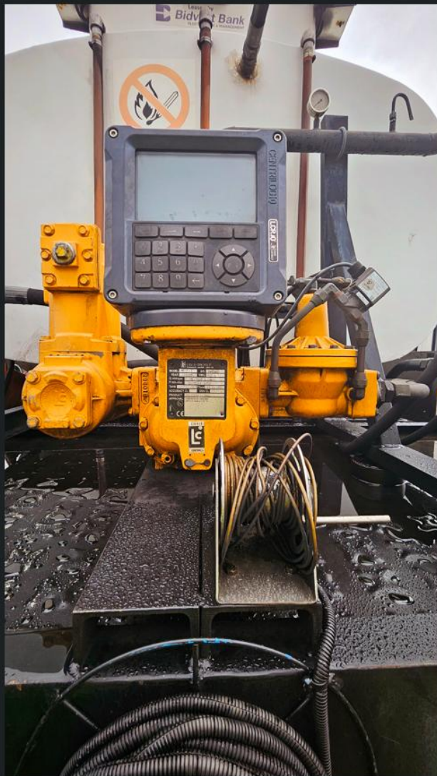
Pier 1 Mobile Bowser Truck - Flow Meter.jpg
