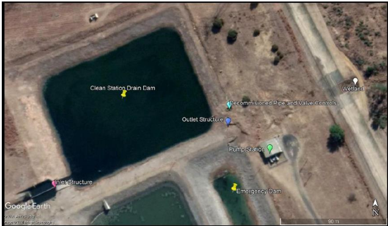
Figure 3: Layout Clean Station Drain Dam
