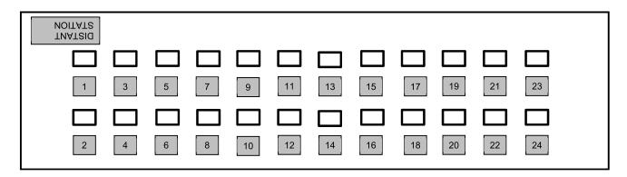
Figure 8: 24-way ODF faceplate labelling
