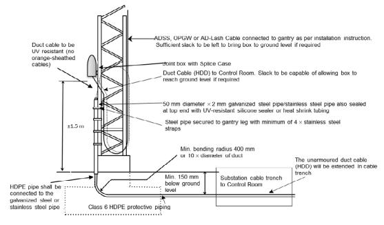
Figure 1: Gantry point fibre connection and termination
