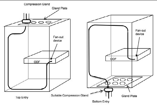
Figure 4: Fibre-optic cable slack routing in cabinet
