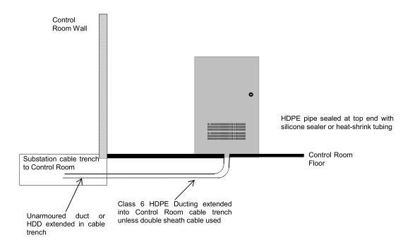
Figure 3: Duct cable arrangements – control room trench termination
