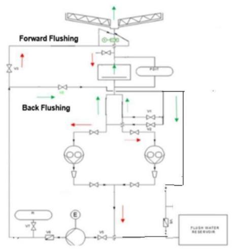
Figure 1: Flushing Modes Schematic.
