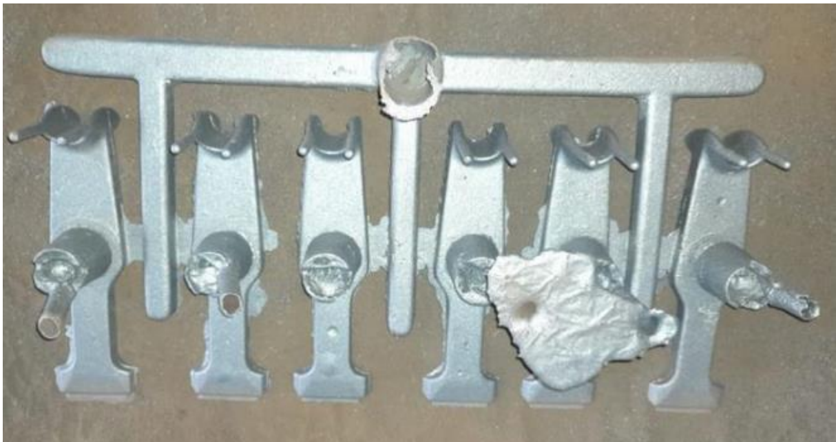
Figure 2: Top view of Centre pieces castings, as received by supplier.
