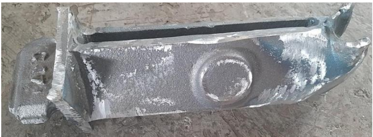
Figure 14: Illustrates the expected Centre piece castings outlook post grinding and dressing.
