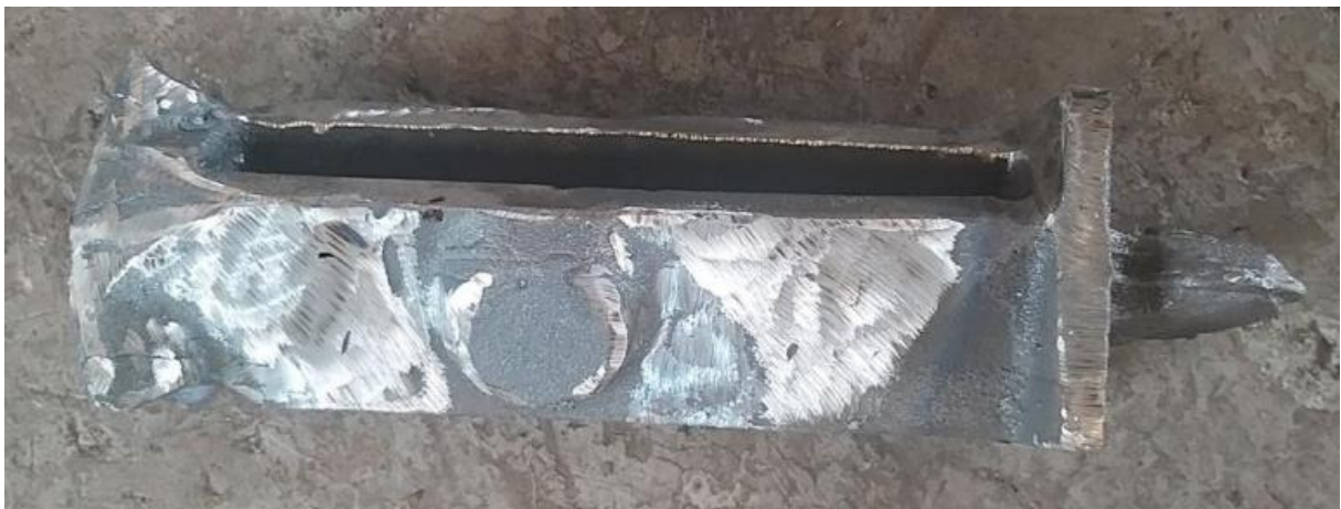
Figure 13: Illustrates the expected Centre piece castings look post grinding and dressing.
