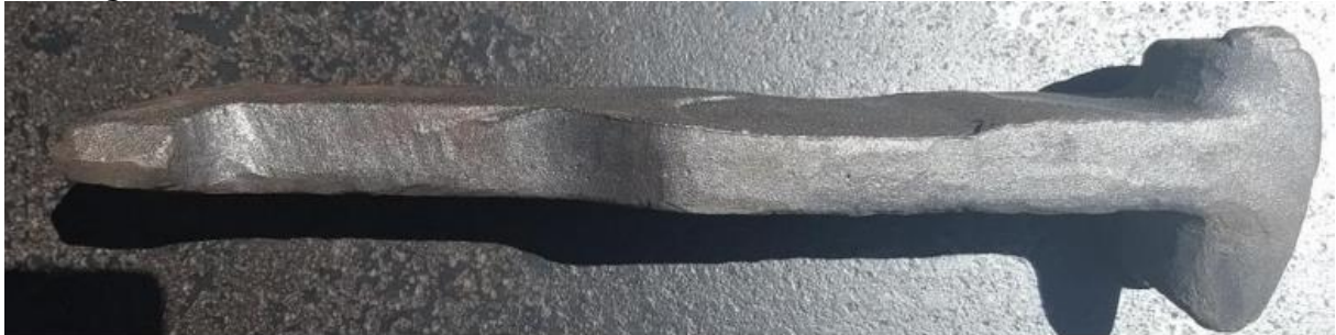
Figure 6: Illustrates top view of a typical KDS Foundry Centre piece casting post grinding and dressing.
