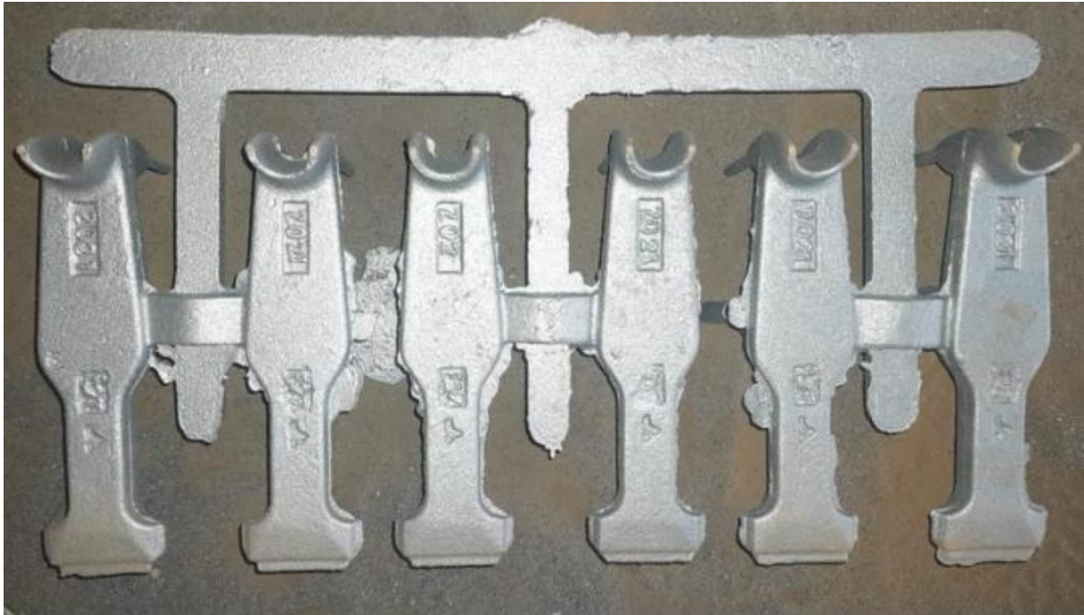
Figure 1: Bottom view of Centre piece castings, as received by supplier.
