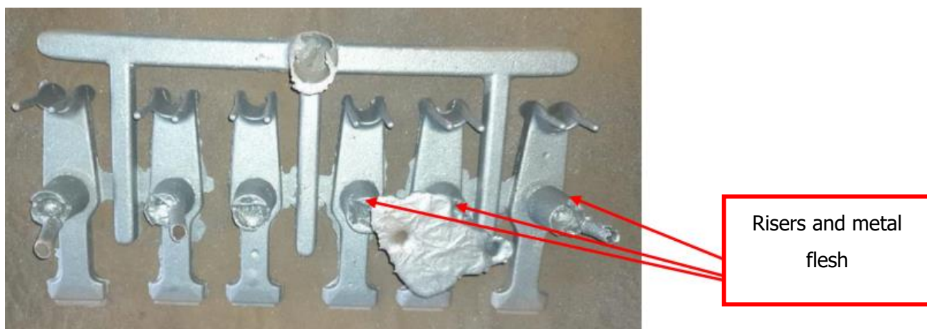
Figure 4: Illustrates the bottom view of Centre piece castings and relevant sections to be cut off.
