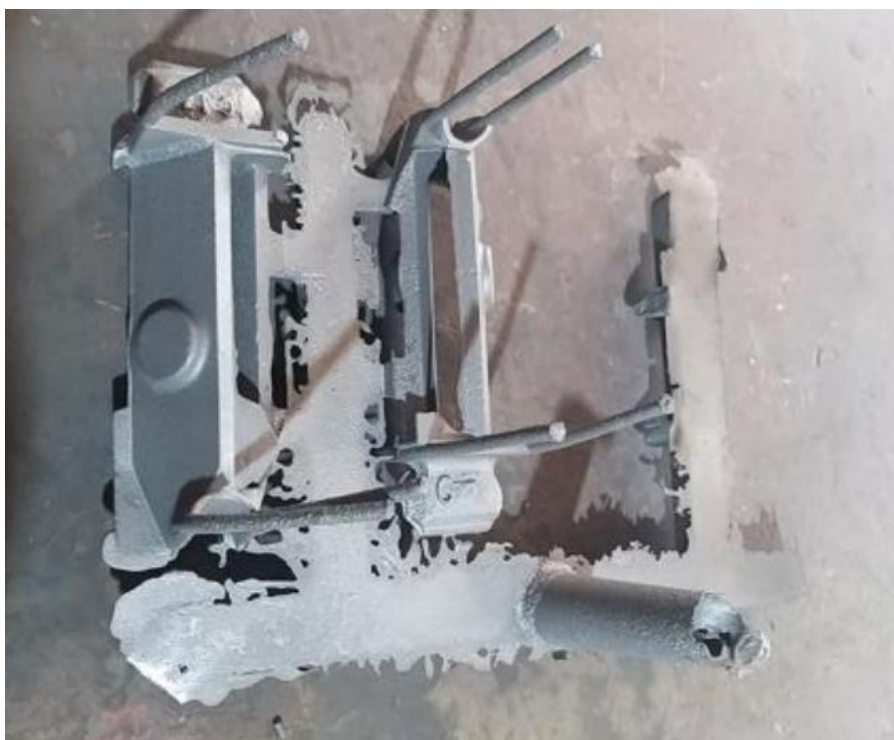
Figure 8: Illustrates the top view of a typical Centre piece casting (set of 4) as received by the supplier.
