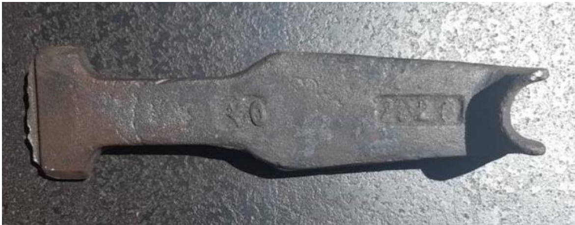
Figure 6: Illustrates top view of a typical KDS Foundry Centre piece casting post grinding and dressing.
