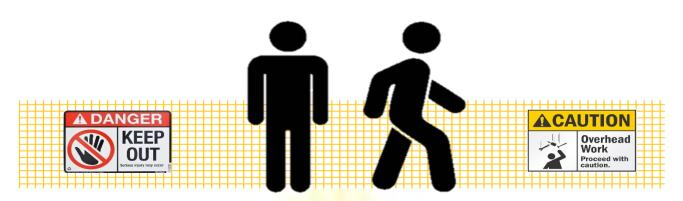
NOTE: Use of danger tapes will <u>NOT</u> be regarded as adequate barricading. PHYSICAL BARRICADING FOR OPEN EDGES AND EXCAVATIONS
