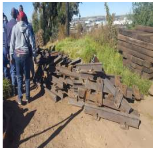
Fig 2.2: Stolen turnout components and sleepers
