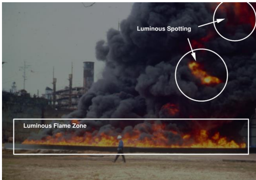
Figure 6: Large hydrocarbon pool fire showing luminous flame region near the base of the fire [112].
