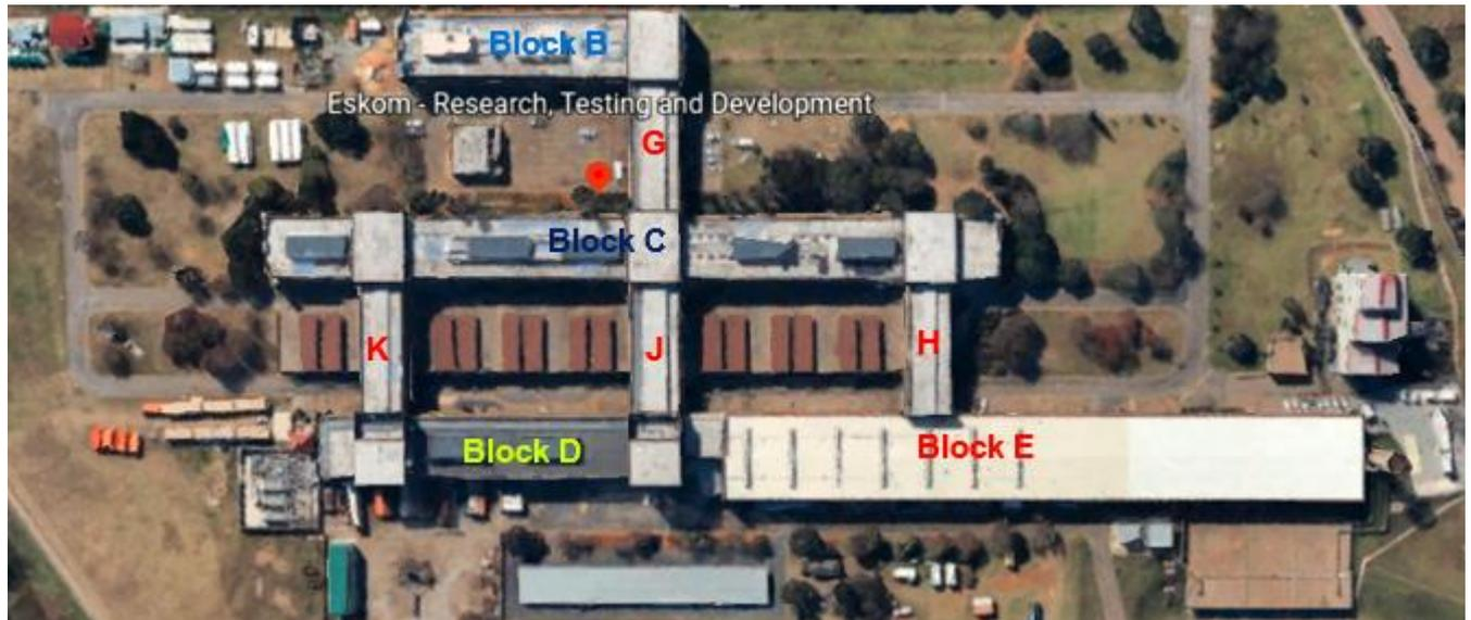
Block E roofing systems comprises IBR sheeting and seven skylight structures. Blocks B, C and D flat concrete slab accessible roofs with water proofing.
