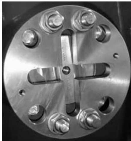
Figure 5: Typical mechanical lockout device
