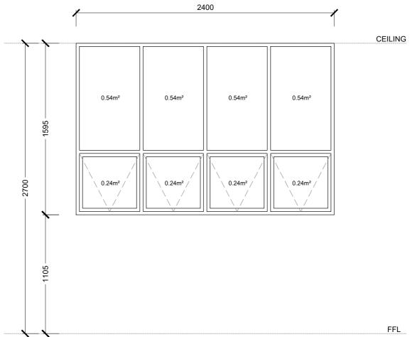
Type. L Crealco Swift 38 or eq. approved top hung aluminium casement window, per layout. Casement sash 1500 x 1200mm max capacity
