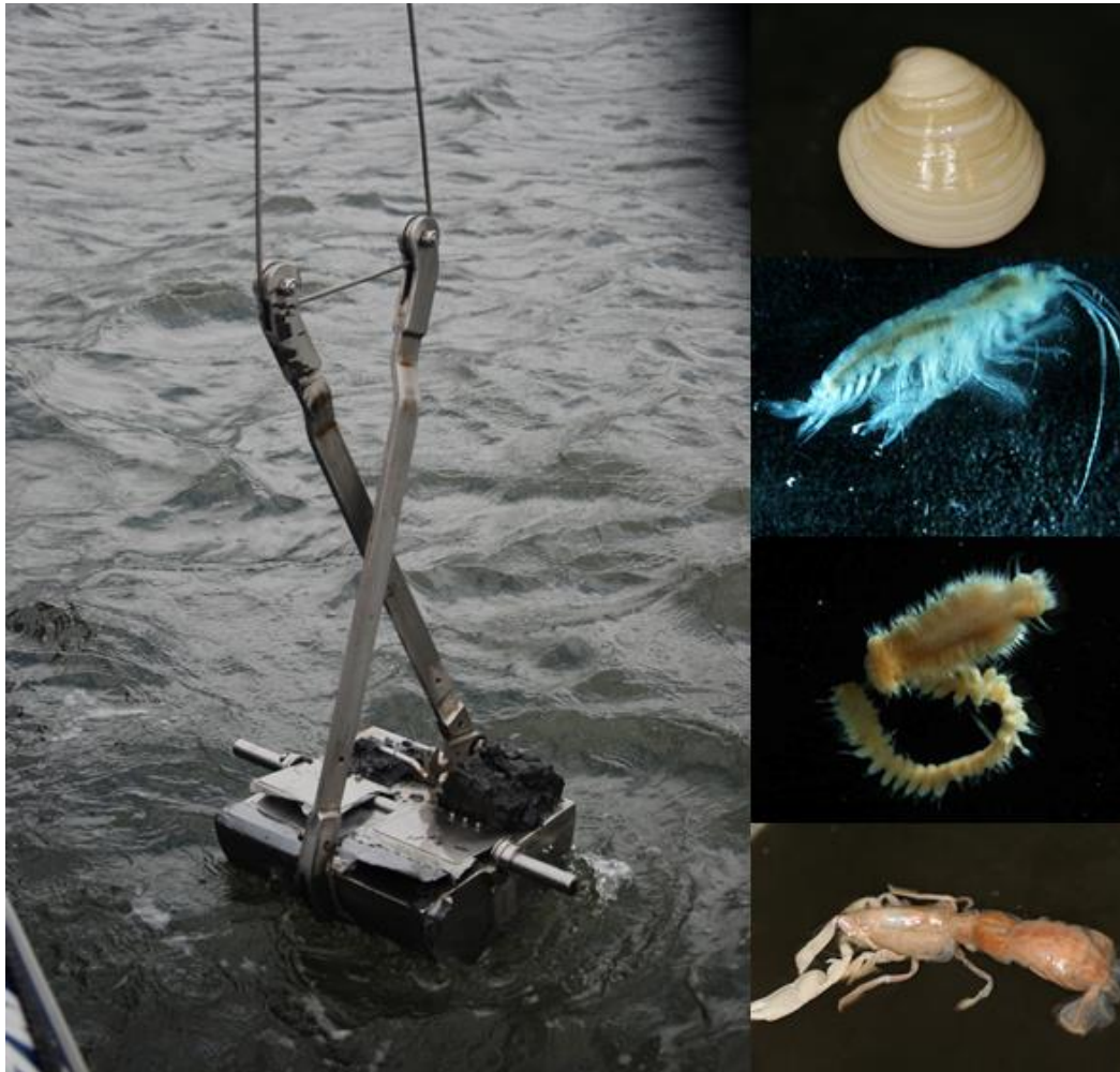
Figure 6.1: Subtidal macrofauna sampling –Grab with sample (left), Examples of macrofauna specimens collected (right).
